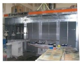
We use only automotive-grade Matthews polyurethane acrylic colors and clearcoats, a proprietary long-lasting metal powder and binder, and MinWax stains. After each coat is sprayed, the sign is placed in a heated drying room to allow the coatings to cure.
